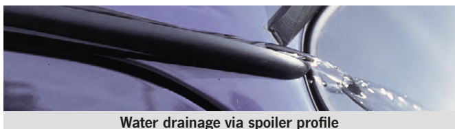
Water drainage via spoiler profile
