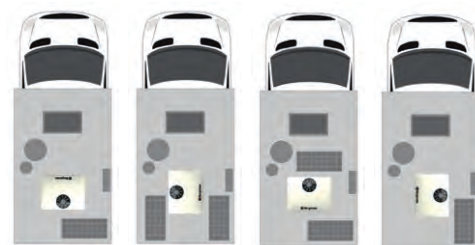
Flexible mounting options: Depending on space available, the outdoor unit can be mounted lengthways or crossways on vehicle roof.
