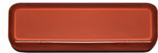
Used in Adria, SEA, Kabe, Atlantis. Homogeneous light emission surface. Fastening with 3M self-adhesive film. 12 V, 1 W, red. 65 x 20 mm, cable 250 mm.
