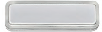
Used in Adria, SEA, Kabe, Atlantis. Homogeneous light emission surface. Fastening with 3M self-adhesive film. 12 V, 1 W, white, 65 x 20 mm, cable 250 mm.
