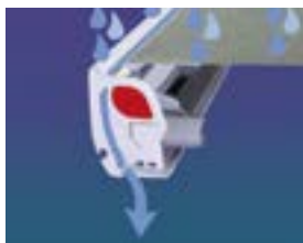
Rain gutter in the front panel diverts rainwater runoff to the sides.
