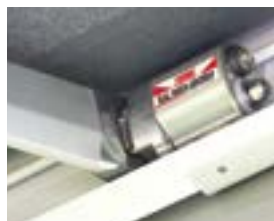
Dual-shock absorbers on the support arms absorb wind movements, for example, and thus protect the awning and vehicle.
